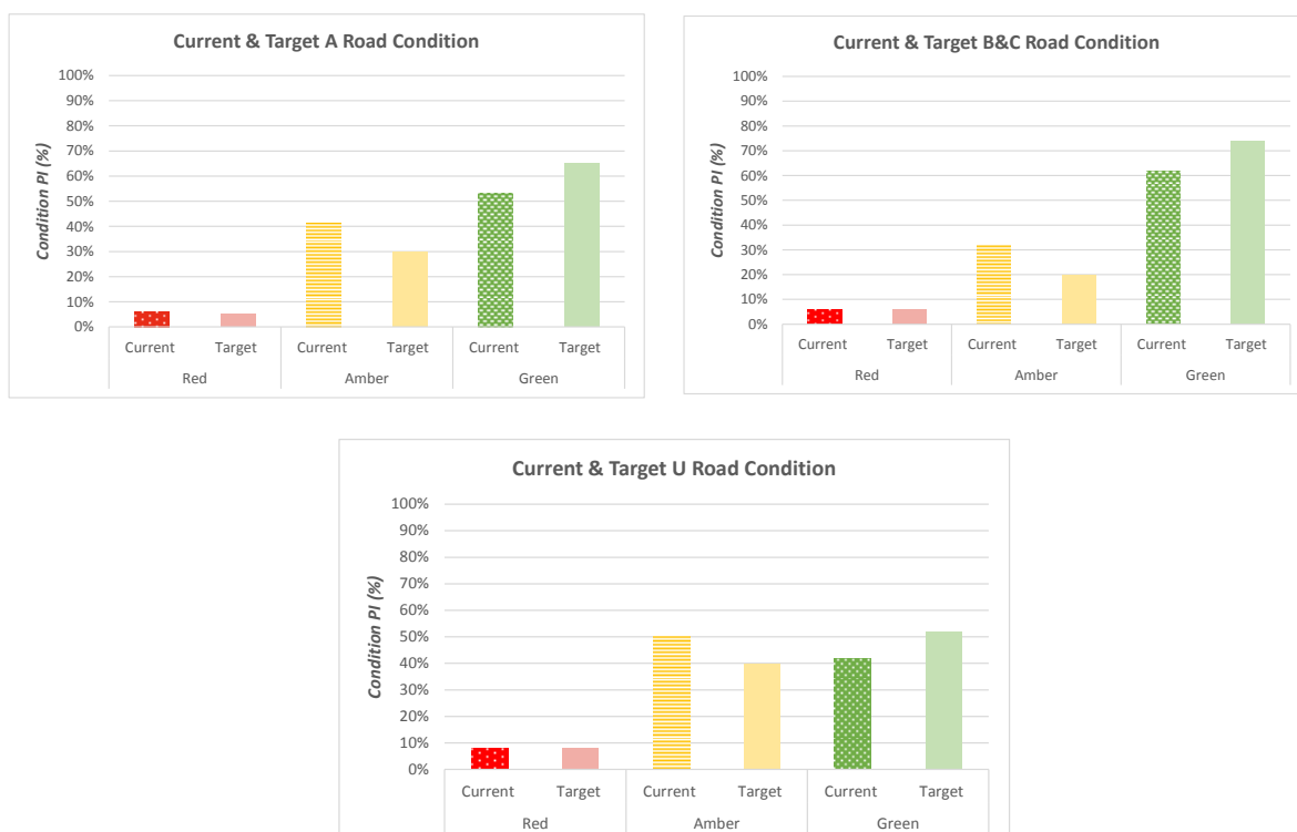
Figure 4: Current and target carriageway surface conditions for A, B&C, and U roads
